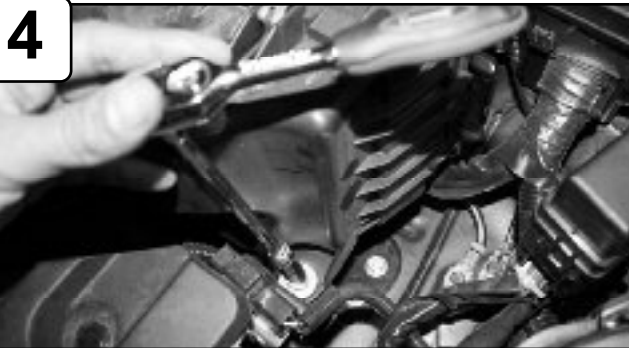
With 10mm socket or wrench loosen the bolt holding bottom half of air box.
