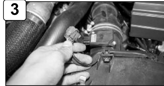
Disconnect MAF sensor harness. Loosen clamp using 10mm socket or wrench.
