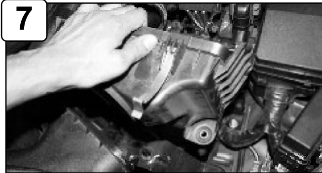
Lift and remove bottom half of air box out of vehicle.
