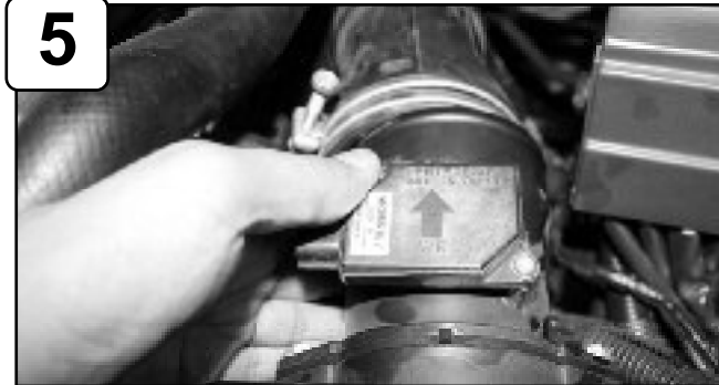
Pull back MAF sensor from intake tube.
