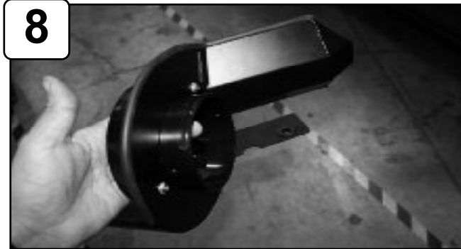
Install filter adaptor to housing and secure using button head screws provided. Tighten using 4mm allen key. Attach rubber trim to top of housing.
