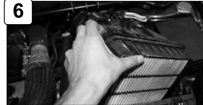
Un-clip upper half of air box and remove.
