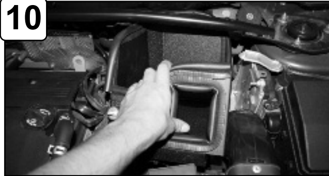
10 Install housing and position grommets on housing to factory fittings.
