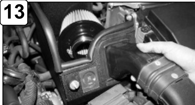
13 Place filter in housing. Attach ram air assembly to housing.
