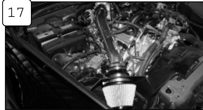
17 Re-install all engine covers. (Intake is shown with no plastic covers on)
