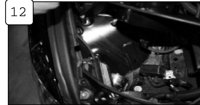
12 Secure housing using provided screws and flat washers and tighten using 10mm socket or wrench.
