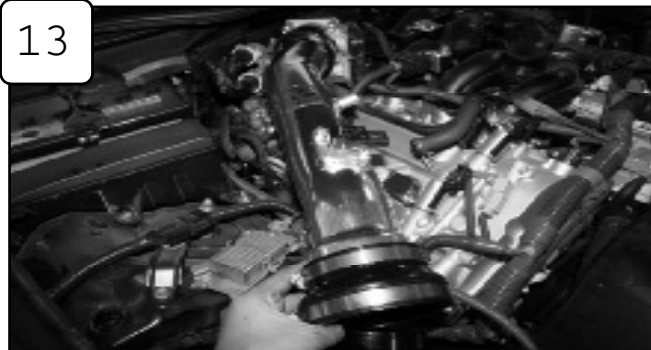
13 Install intake tube with couplers and clamps provided. Do not tighten.
