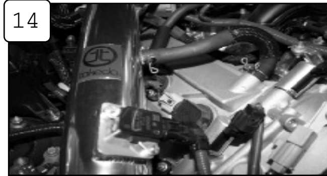
14 Re-connect MAF sensor harness and crank case line.
