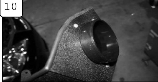
10 Attach adaptor to housing using button head screws provided. Attach trim seal to top of housing and cut out for scoop.
