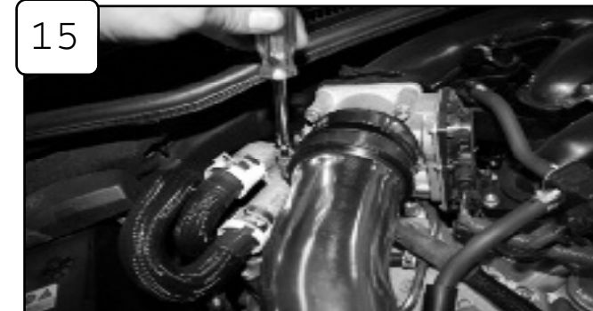
15 Tighten all clamps using 5/16" nut driver.
