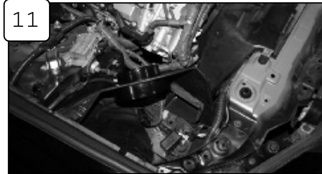
11 Position housing in the engine compartment.
