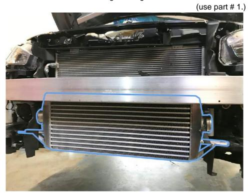
2.3 Insert the provided M10x40mm bolt(s) through the lower under frame through both sides of the factory intercooler rubber bushings and new Intercooler brackets. \*(Some early kits will have a pre-welded stud that fits into the factory rubber bushing from above, instead of the provided #10. bolt.)
