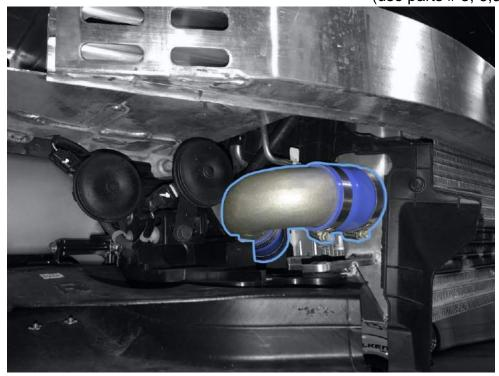
2.5 Next install the other "hot pipe" I-1 in between the factory turbo outlet and the lower pipe I-2 you just installed.
