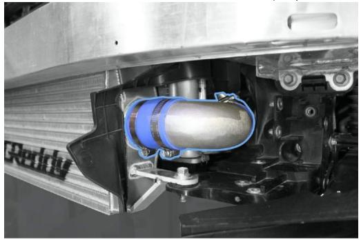
2.8 Align the all of the intercooler piping for proper clearance and tighten all hose clamps.
