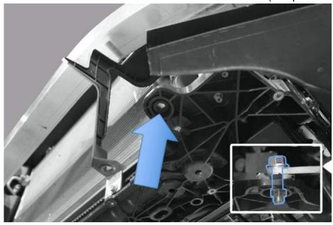
2.4 Connect the lower "hot pipe" I-2 to the intercooler.
