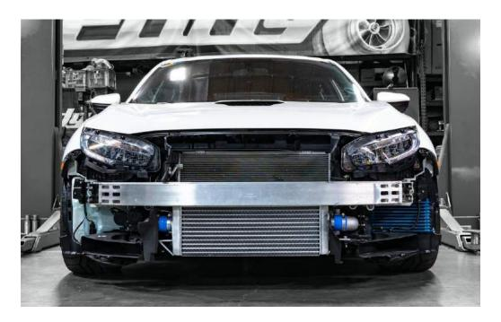
2.9 Before reinstalling the bumper and lower under cover, some of the inner structure of the lower undercover will have to be trimmed as shown below. Be sure to cut a little at a time, until the lower panel just fits over the intercooler without interference.
