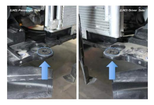
2.2 Slide in the new Intercooler into place, behind the bumper support and let it rest on the stock intercooler mounting bushings.
