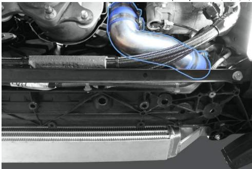
2.6 On the other side of the intercooler, loosely install the I-4 intercooler piping onto the factory upper intercooler pipe.
