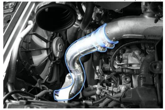
2.7 Next, install intercooler pipe I-3 in between the Intercooler and intercooler pipe I-4, that you just installed.
