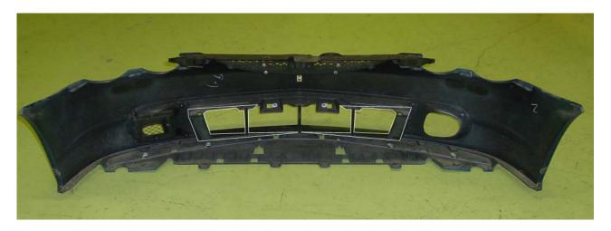
Cut the bumper little by little and test fit on the vehicle. Trim the area the hits the \* intercooler.
