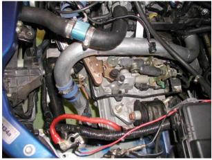
(3) Install the I-3 pipe between I-2 and intercooler inlet as shown.(Parts Used #: 4, 12, 14)
