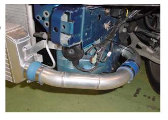
(4) Install the I-4 to the intercooler outlet as shown.
