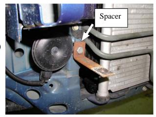
(2) Mount the Intercooler shown using provided hardware. Secure the left side of the intercooler (looking from the front of the vehicle) to the bracket installed in the previous step.
