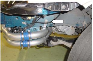
(6) Install the Compression pipe C-3 from the turbo kit between the pipe I-5 and the throttle body as shown. Reuse the hoses and clamps from the turbo kit.
