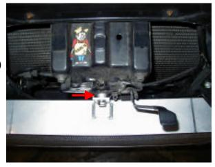
(2) Mount the bottom bracket of the inter cooler to the sub-frame using the provided hardware as shown.
