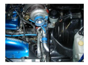
(3) Install the I-2 pipe between the I-1 and the intercooler as shown.
