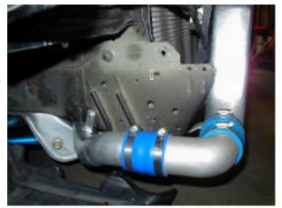
(5) Install theI-5 and I-6 using provided hose and hose band as shown. Install the 16 hose to the I-6 and the idle air control valve as shown.
