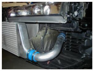
(4) Install thel-3 and I-4 using provided hose and hose band as shown. Secure the bracket on the I-4 pipe to the body as shown.
