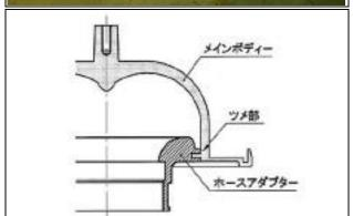
(2) Install the Airinx and the airflow meter on to the suction pipe as shown.
