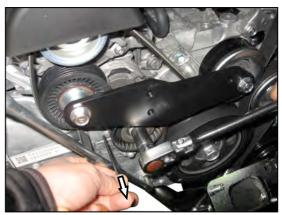
(4) Install the Turbo assembly, and install the turbine inlet gasket.
