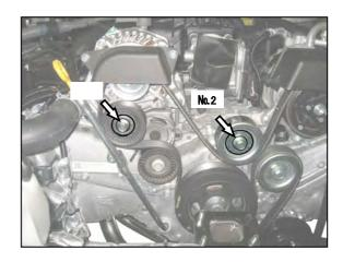
When installing the Turbo Mounting Bracket, be sure to not remove the serpentine belt.
