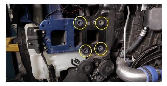
3.3 Place the block off panels over the large holes and screw the two remaining M8 bolts into the chassis like in the pictures below.
