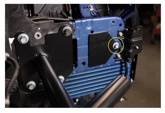
3.4 If you are using the GReddy side mount oil cooler or transmission cooler then you will need to use the vibration loop clamp to attach to the air diversion panel. Slip the clamp over the bar with the flat side of the clamp facing forward. Using the M5 bolt and nut, secure the diversion panel to the vibration loop clamp.
