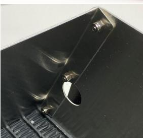
19. Mount the cooler core to the chassis as shown (ITEM #19, 21, 24).
