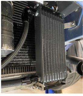
Attach hoses from engine block adapter to oil filter relocation adapter (ITEM #10, 11).
