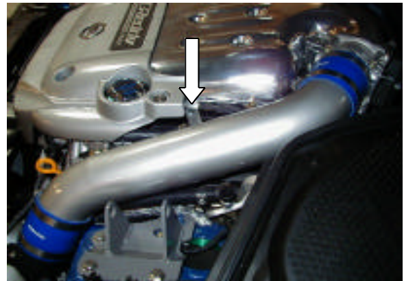
Secure the bracket on C-6 to the Intake manifold
