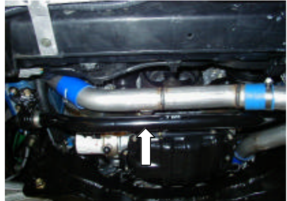
Secure the bracket on C-3 to the block
